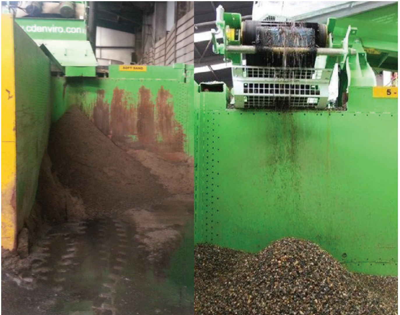
Sand and gravel recycled from Hertfordshire's street sweepings
